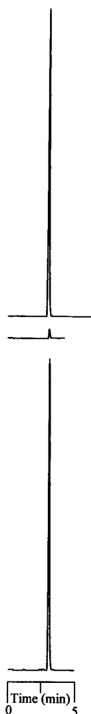
Figure 1. Chromatograms showing the adsorption of diphenyl phthalate (compound 2 in Table 1) before (bottom) and after (center) the process was completed in hexane. The percentage of adsorption was estimated to be 96.8% for a time period of 1 h. However, the adsorption was not observed in acetonitrile, as shown in the chromatogram on the top. Refer to Table 1 for chromatographic conditions and recovery rate.
